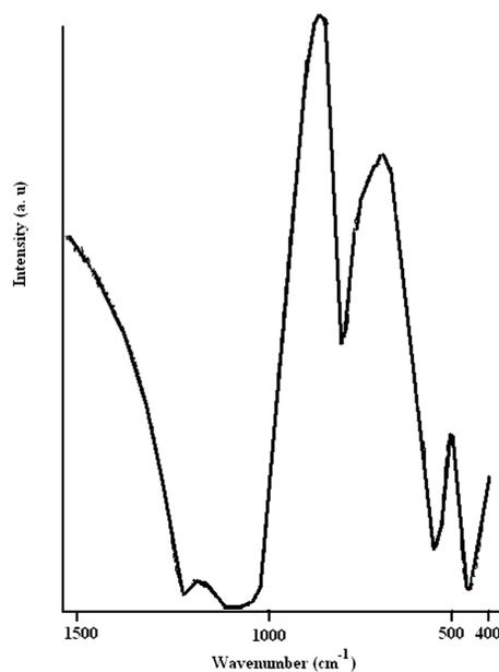
**Figure 2,** FT-IR spectra of calcinated ZSM-5 zeolite
