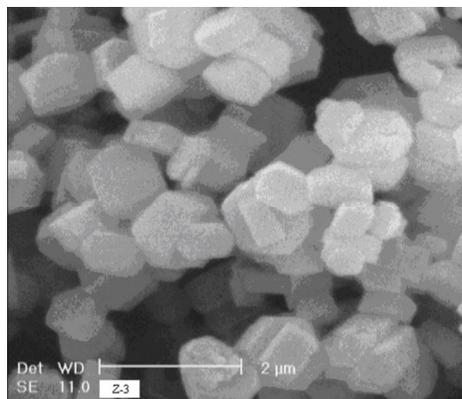
**Figure 4.** SEM image of the synthesized ZSM-5 crystallites
