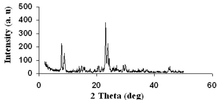
**Figure 3.** X-ray diffractogram of the as-synthesized ZSM-5 zeolite.
