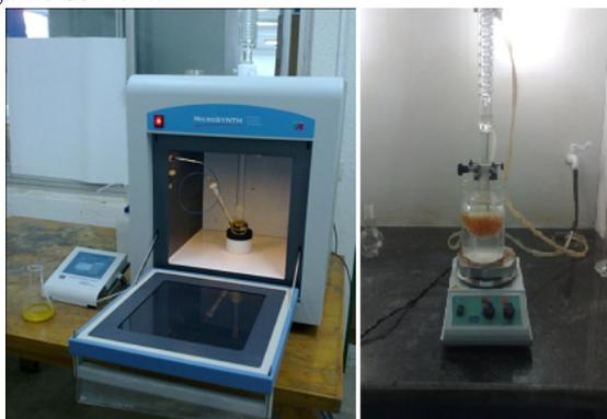
Figure 1: Microwave reflux system and Reflux by oil bath
