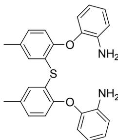
**Fig 1.** Chemical structure of 2, 2'-thio-bis [4-methyl (2-amino phenoxy) phenyl ether) (TBMAPPE).
