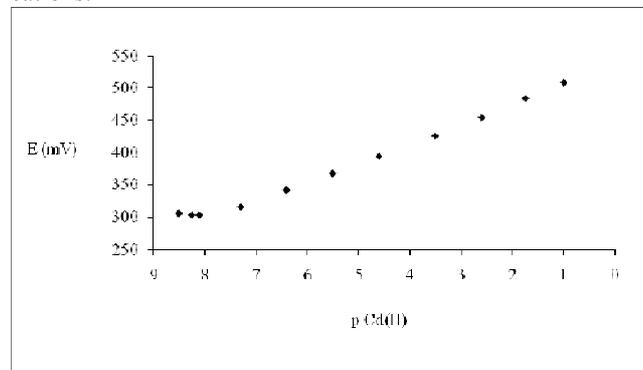
**Fig. 3.** The calibration curve of the Cd<sup>2+</sup> nano-composite carbon paste electrode (No. 10).
