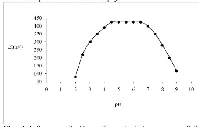
**Fig. 4** Influence of pH on the potential response of the cadmium-selective electrode  $1.0 \times 10^{-3} \text{ mol L}^{-1} \text{ Cd}^{2+}$ .
