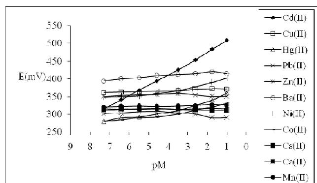
**Fig. 2.** Schematic diagram of electrode response to various cations.
