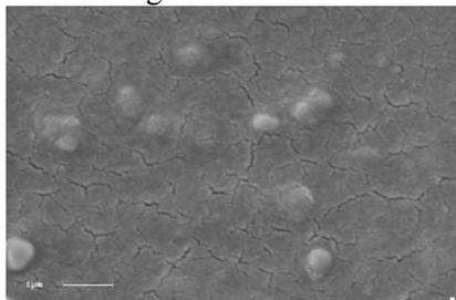
**Figure 1.** SEM micrographs of Nylon6/Poly (butylene terephthalate) blend containing 20% PBT without appropriate compounding system
