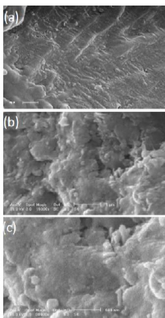
**Figure 2.** SEM micrographs of the Nylon6/Poly (butylene terephthalate) blend containing 40% PBT with appropriate compounding system at three different magnifications
