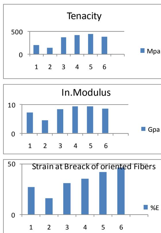
**Figure 7.** Tensile properties of hybrid blend fibers
