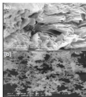
**Figure 3.** SEM micrographs of the Nylon6/Poly (butylene terephthalate) blend containing 30% PBT (a) before being etched, (b) after being etched
