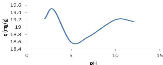
**Figure 3:** The effect of pH on the removal efficiency with: PANi/AC (The initial concentration, contact time, volume of solution and amount of adsorbent was 20 mg/L, 60 min, 100 mL and 0.1 g, respectively).
