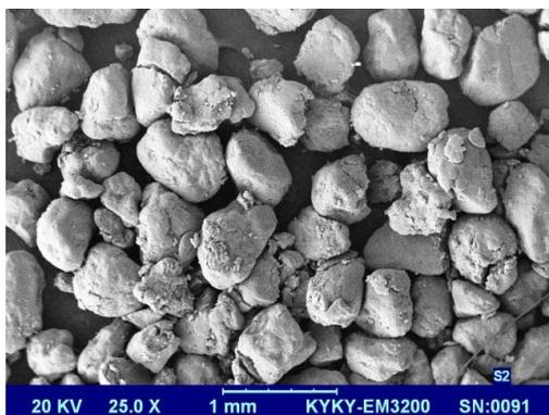
**Figure 1:** SEM image of activated carbon
