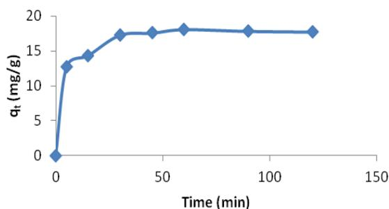
**Figure 5:** The effect of contact time on the removal efficiency with: PANi/AC (the initial concentration, pH, volume of solution and amount of adsorbent was 20 mg/L, 3, 100 mL and 0.1 g, respectively).
