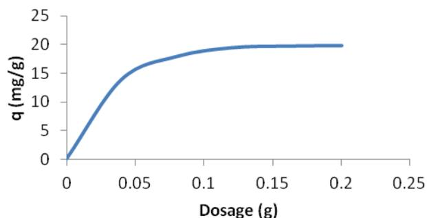
**Figure 4:** The effect of adsorbent dosage on the removal efficiency with: PANi/AC (the initial concentration, pH,
