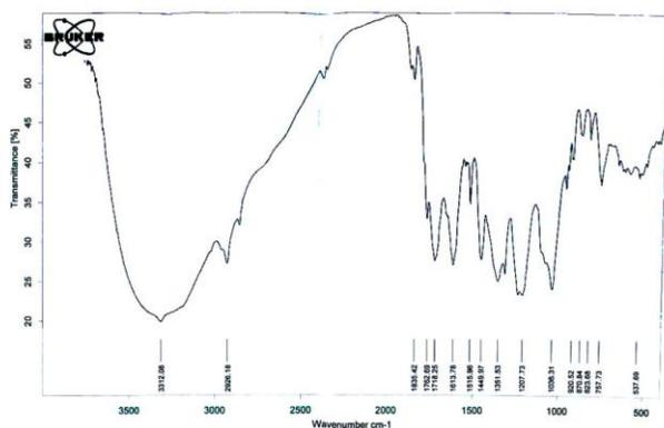
**Figure 3:** FT-IR spectrum of silver nanoparticles synthesized with Water lily flower
