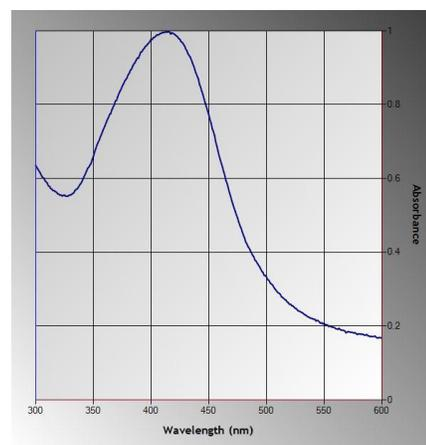
**Figure 4:** UV-Vis spectrum of biosynthesized silver nanoparticles.
