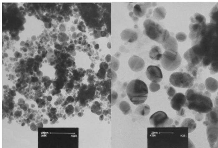
**Figure 1:** TEM micrograph of Ag NPs synthesized with Water lily flower extraction.
