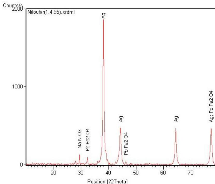
**Figure 2:** XRD of Ag NPs synthesized with Water lily flower extraction.
