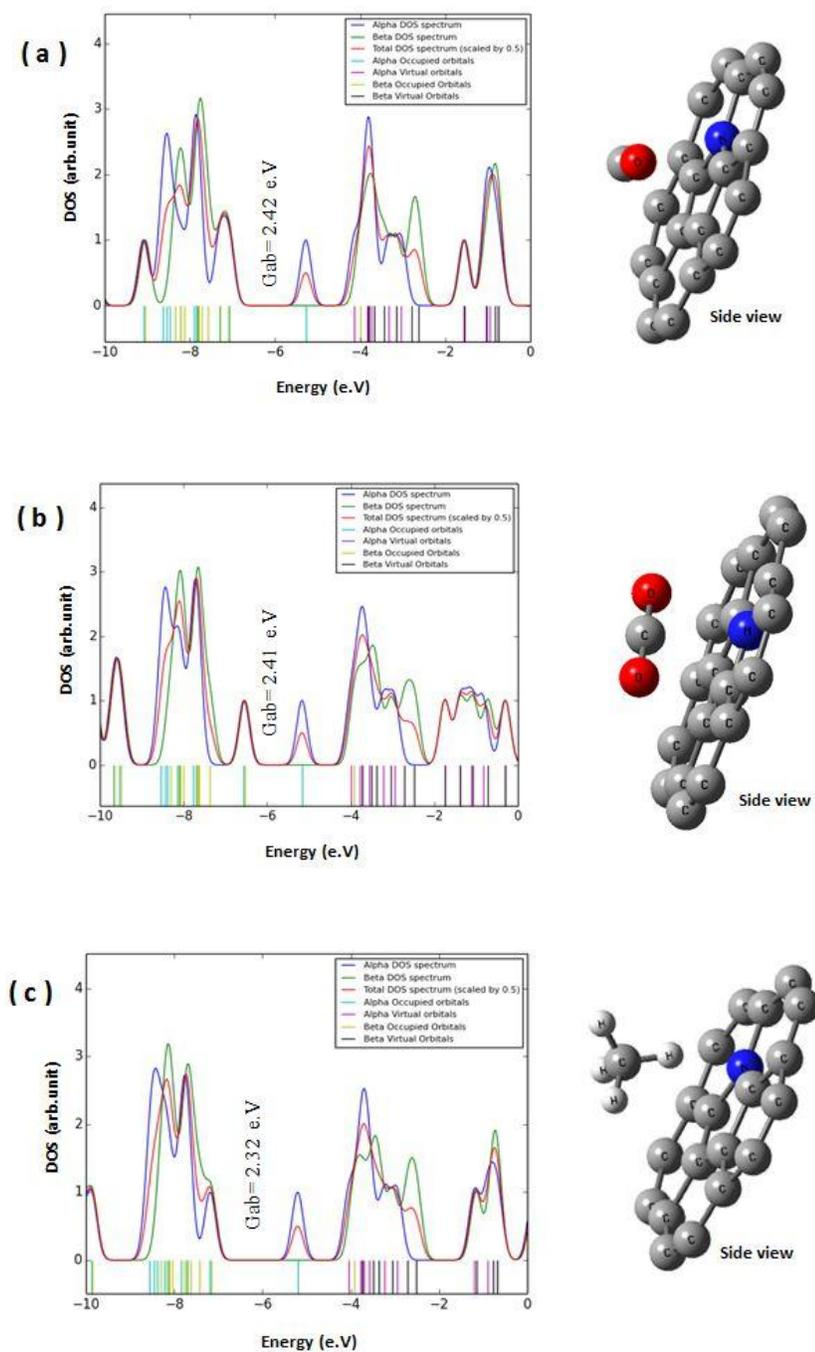
**Figure3:** the optimized structure of gas molecules (a) CO, (b) CO<sub>2</sub>, (c) CH<sub>4</sub> adsorbed on N-doped fullerene and its densityofstates (DOS).
