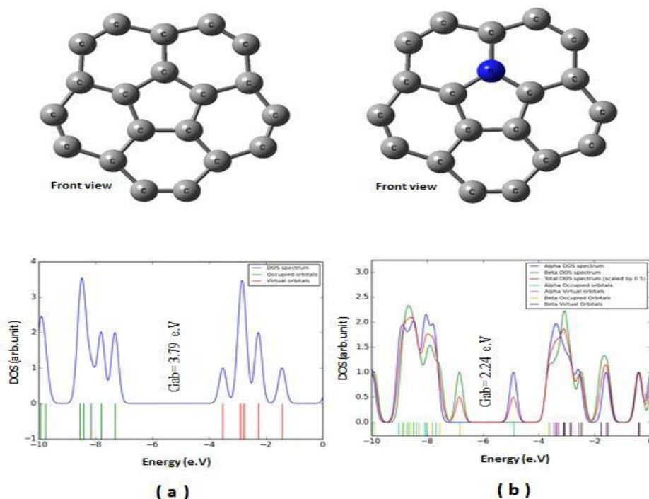
**Figure 1:** the optimized structure of (a) pure fullerene bowl and (b) N-fullerene and its density of states (DOS).
