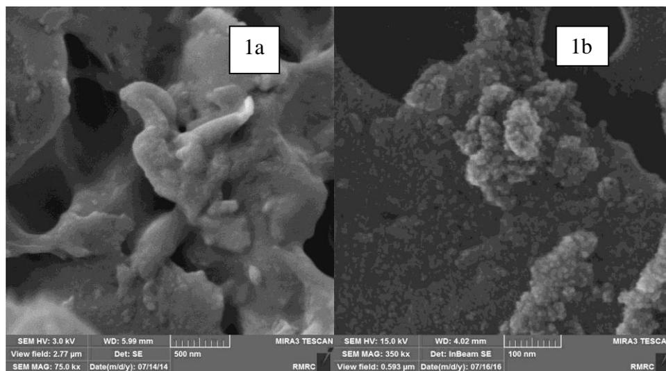
**Figure 1:** (a) SEM micrograph of sawdust (b) SEM micrograph of nano-sawdust-OSnCl<sub>3</sub>
