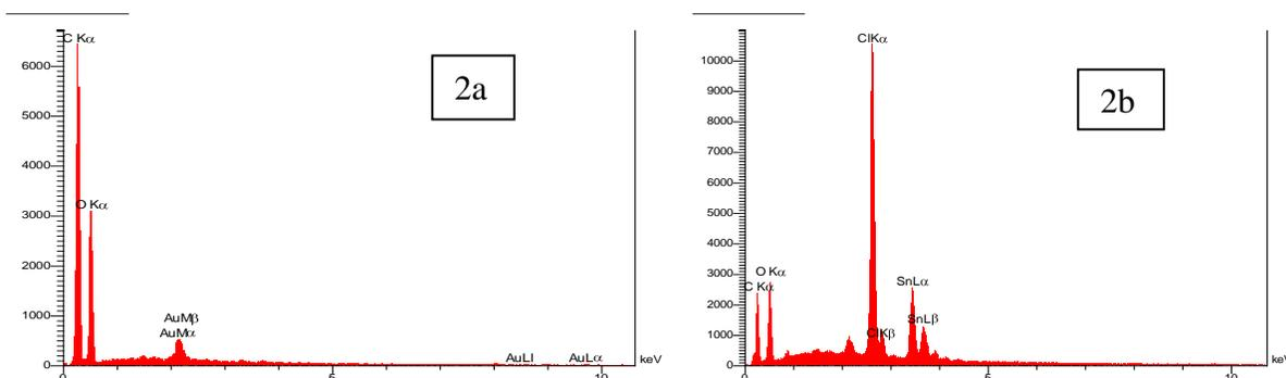
**Figure 2:** (a) EDX of Sawdust and (b) EDX of nano-sawdust-OSnCl<sub>3</sub>
