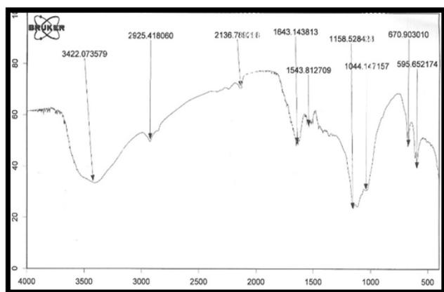
**Figure 3:** FT IR spectrum of nano-sawdust-OSnCl<sub>3</sub> catalyst
